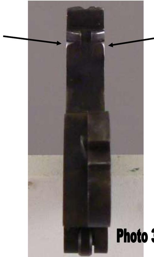
It isn't necessary (or possible on some guns) to completely remove all side-to-side hammer contact. What we want is a smooth transition in the event the hammer happens to rub on the frame while shooting. Once the hammer moves smoothly in the frame, we will move on to the most critical part of our tune-up--fitting the cylinder bolt to the cylinder.
