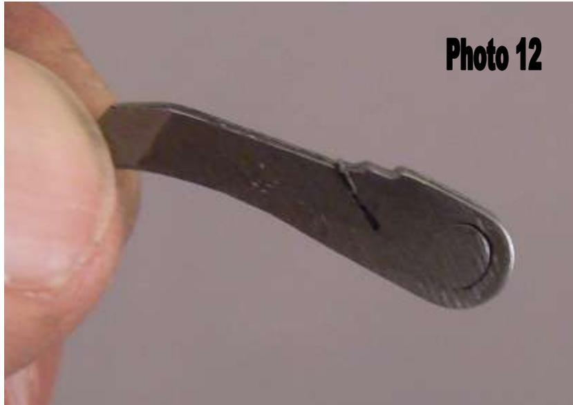
Now that it's broke, we'll fix it permanently. For this step, do not try to remove the broken-off stub. We want it in the slot. With the hand spring gone, you can see how rough the back of the hand is. Photo 13.
