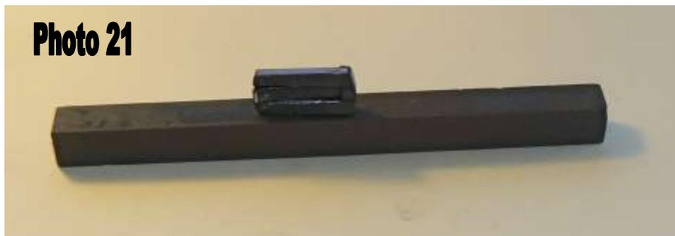
Repeat the process on the second side of the wedge, testing frequently, until the tip of the wedge spring just sticks out of the barrel with thumb pressure on the wedge. Photo 22.
