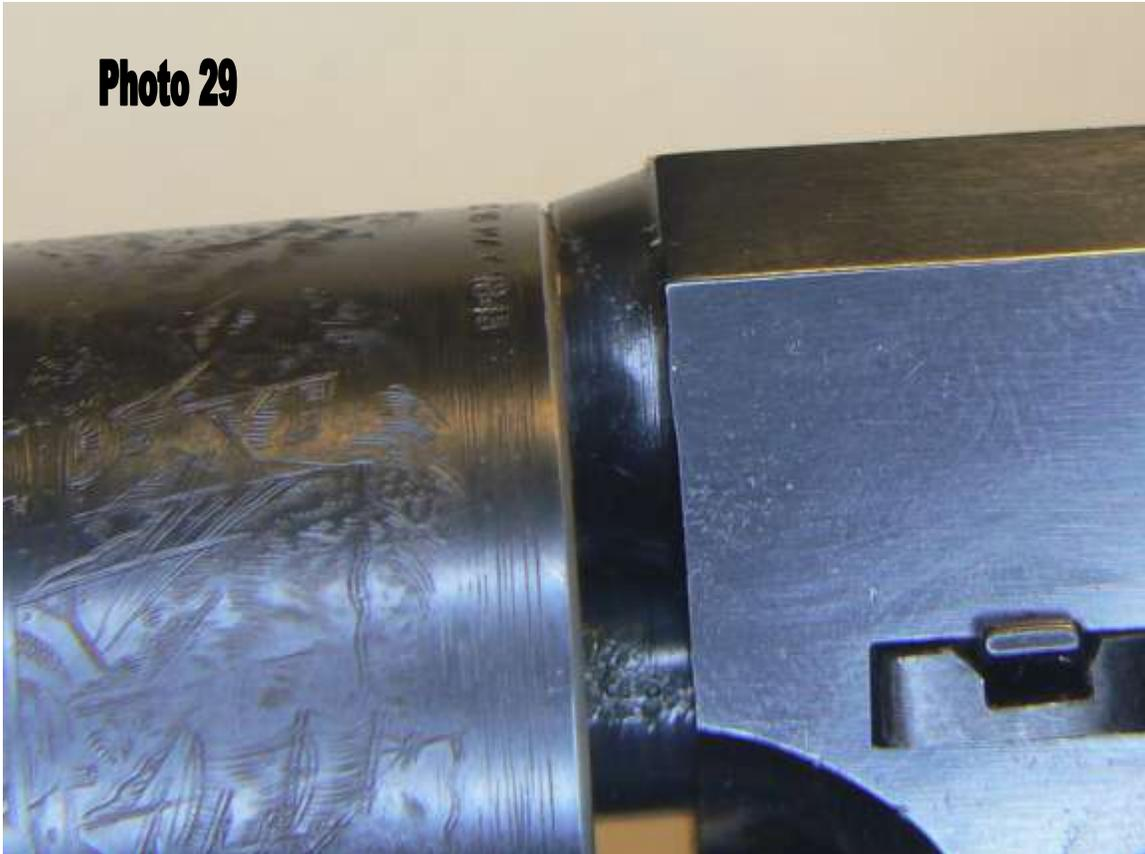
When firing, the front of the cylinder gets dirty and it will drag more and more on the back of the barrel as more shots are fired. Use good grease over the balls to help keep the fouling soft and/or wipe the face of the cylinder off every couple of stages.
