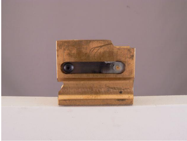
Photo 12 (above) shows a carrier modified with what is functionally a miniature-loading gate milled into the side of the carrier. As rounds push past the gate they sit on a tab that holds them toward the front of the carrier. With rounds held at the front of the carrier,
