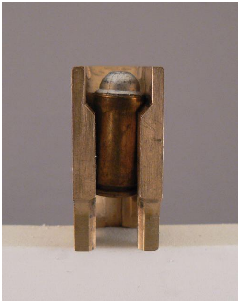
Photo 12 (above) shows a carrier modified with what is functionally a miniature-loading gate milled into the side of the carrier. As rounds push past the gate they sit on a tab that holds them toward the front of the carrier. With rounds held at the front of the carrier,
